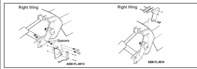
Remove belt guard. Assemble the rod end of the tilt cylinder. Use the pin located in the ears on the end of the housing and secure with the cotter pins. Reinstall belt guard.
